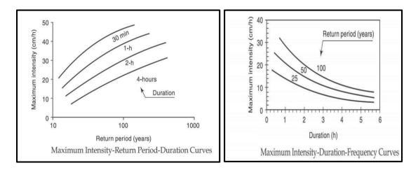
Suppose one has to determine the design discharge of a storm sewer with a consideration that its return period is not less than 5 years i.e., the risk of storm sewer getting over flooded is acceptable once in 5 years.
